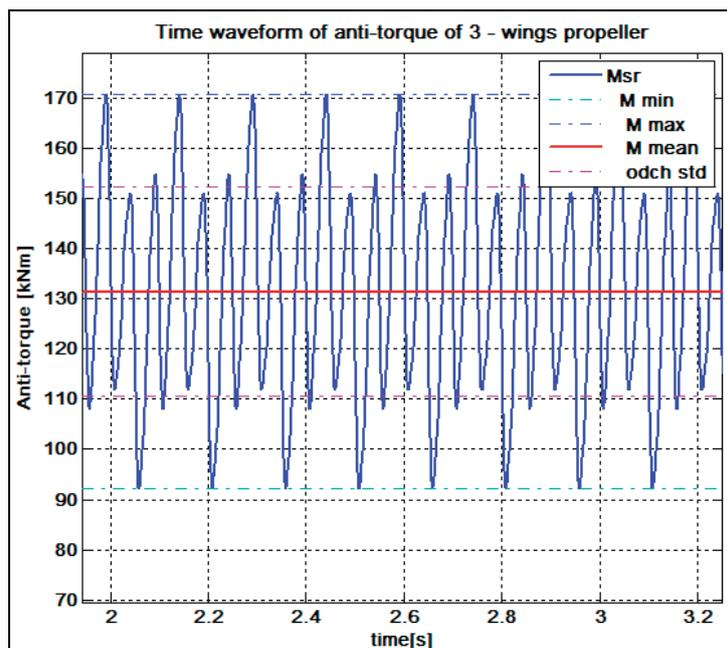
Fig. 5. Simulations of time waveform of anti - torque,  $M = 35\%$  load
