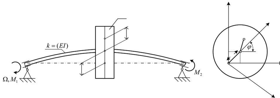
Fig. 1. A simplified shaft-line model for critical speed calculation [3] where:  $M_1$  - torque,  $M_2$  - anti-torque
