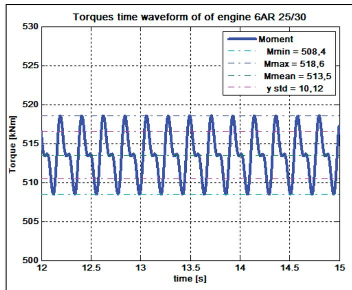
Fig. 4. Simulations of time waveform of driving torque,  $M = 100\%$  load
