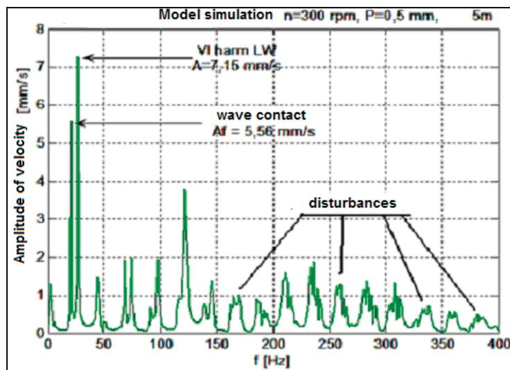
Fig. 8. Average spectrum of velocity,  $n = 300$  rpm,  $e = 0.5$  mm, wave amplitude 5 m (model)
