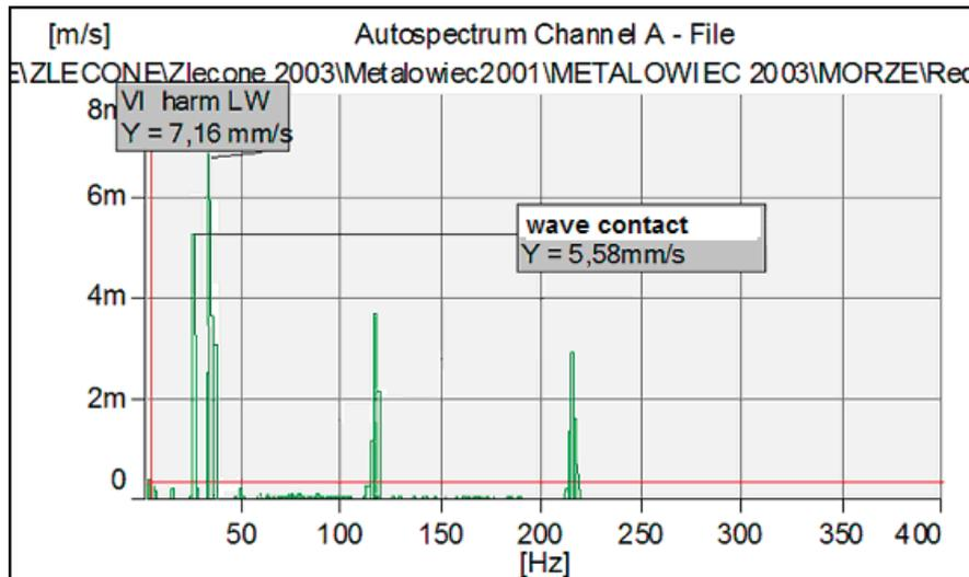
Fig. 9. Average spectrum of velocity,  $n = 300 \text{ rpm}$ ,  $e = 0.5 \text{ mm}$ , wave amplitude 5 m (real object)
