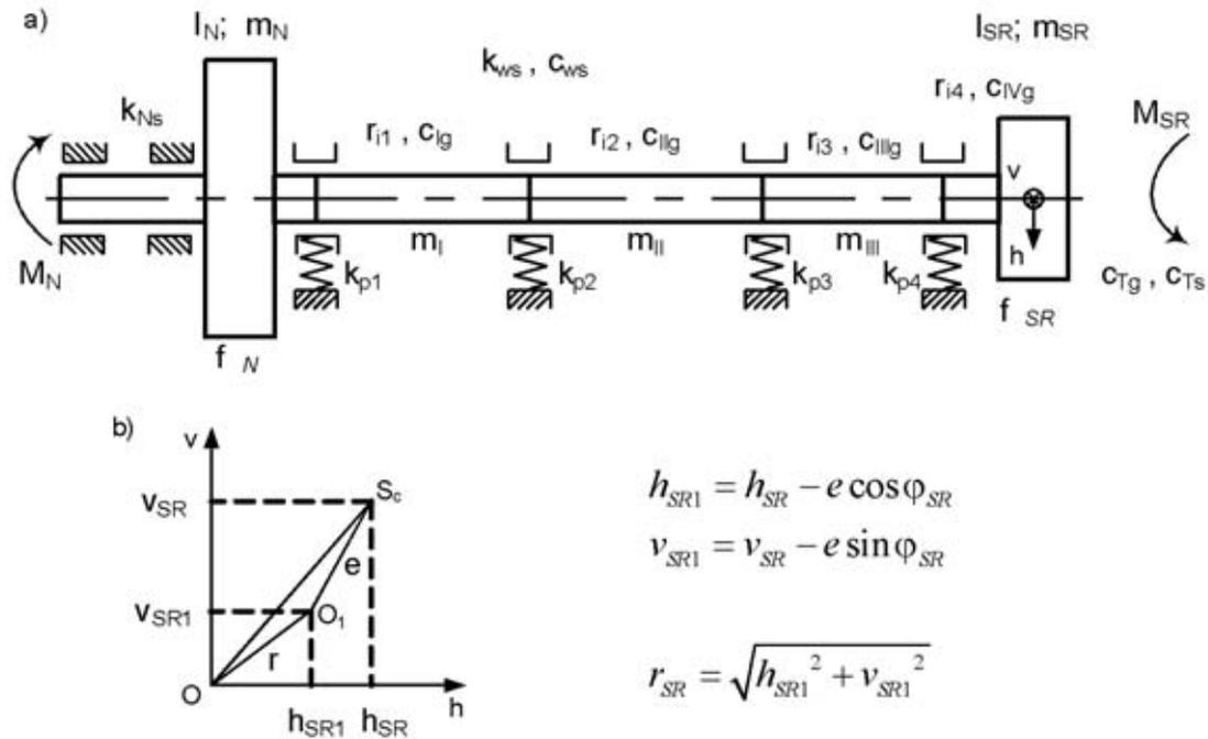
Fig. 2. Model of excitation of propeller shaft for simulation process where:  $I$  - moments of inertia,  $m$  - masses  $k$  - coefficients of stiffness,  $c$  - coefficients of damping,  $N$  - drive,  $SR$  - propeller,  $h$  - horizontal axis,  $v$  - vertical axis  $r$  - deflection of support,  $e$  - eccentricity of rotational shafts axis
