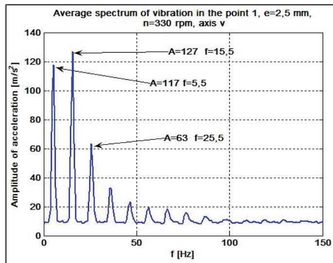
Fig. 7. Average spectrum of acceleration,  $n = 330$  rpm,  $e = 2.5$  mm
